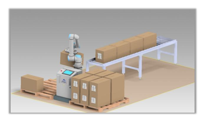
The MPS system is a turn-key palletizing solution that provides end-users the features needed to quickly setup a robot for palletizing cases or other standardized products for final shipment.
